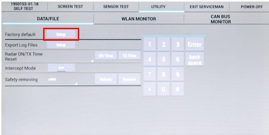
7. When the reset menu appears, touch the pull-down arrow and select "Factory Default (Delete All Settings)" **WARNING:** You are about to clear the unit. Ensure you have backed up any desired user data!!
