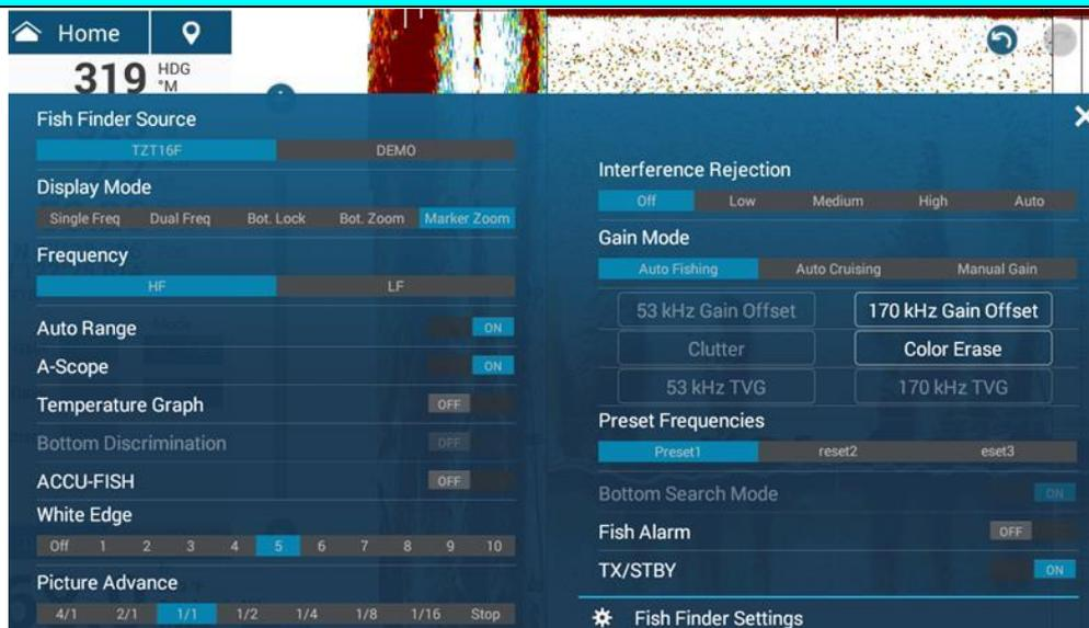
**Display Mode**, **Frequency**, **Auto Range**, and **Gain Mode**, which were selectable in the contextual menu are available in the Layer menu. The new **Preset Frequency** ([Section 3.2](#)) and **Bottom Search Mode** ([Section 3.10](#)) are also accessible from the Layer.
