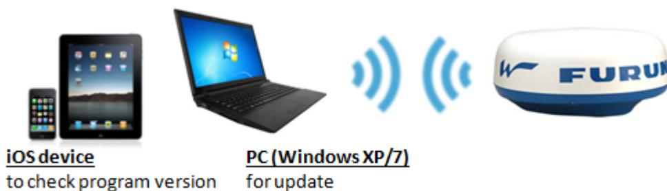
3. Before attempting the software update with the PC, establish communication between the iOS device and the DRS4W as follows.
