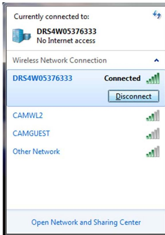
15. Launch the Marine Radar App on the iOS device and connect it to the DRS4W.
