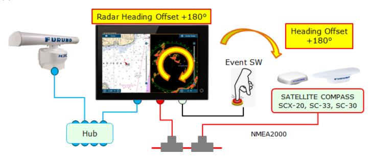
(3) On the TZT12F/16F/19F, or TZtouch2, access [Settings] – [Initial Setup] – [Event Input Configuration] and select [Ferry].
