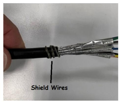
Now carefully wrap all three shielding wires with the conductive tape:
