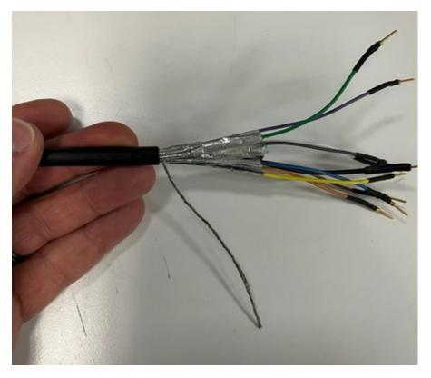
Pick out the three shielding wires, and then wrap these back along the sheath:
