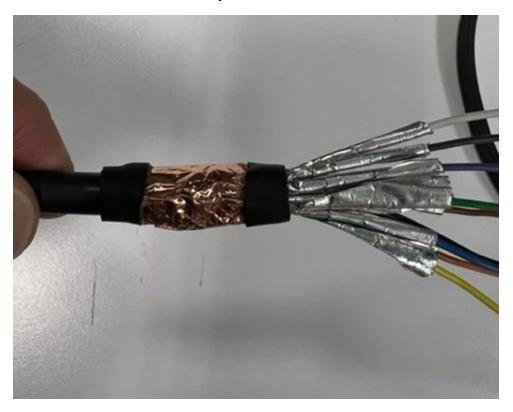
Now carefully install the DFF3D Transducer Wiring into the DFF3D Module:
