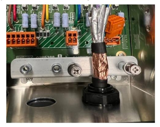
Use the DFF3D grounding clamp to hold the DFF3D Transducer in place where the conductive tape is. This will provide a solid ground for the DFF3D Transducer Wiring to prevent any noise. Also, ensure to connect an Earth Ground to the DFF3D's Grounding Stud to combat any potential noise issues:
