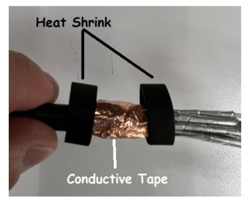
Carefully use a heat gun to apply heat to the heat shrink that will hold the conductive tape in place:
