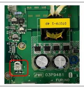
Ensure Jumper is inserted in J7 to bypass Power Synch or PSU will not turn on.
