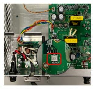
PSU013/PSU012 new out of the box will not have a jumper inserted in J7
