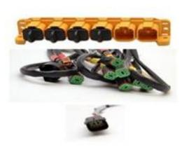
(3) Disconnect the multi-link cable connector and install the Y-split cable for multi-link cable installation or if there is a hub simply plug the Helm Master gateway into the open port on the hub and disregard the Y-Split Cable. NOTE: There will be several similar style bus connectors but only the correct ones will fit properly.
