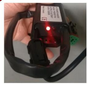
Check the incoming data to make sure that the three proprietary PGNs coming from the gateway are in black. If they are light grey there is a problem with the network. Check to make sure you have a red light on the gateway. Make sure you have a proper CAN bus network, such as 2 terminating resistors.
