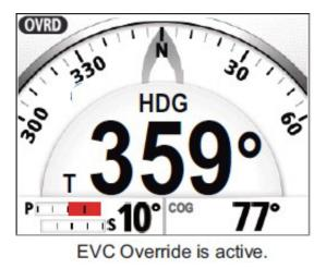
**Note:** Two rudders are controlled separately during Optimus operation modes. Consequently, the Optimus PCM alternatively outputs two rudder angles. The NavPilot will toggle the display of the rudder angles during Override (OVRD) mode. The following photo shows how operation modes of the Seastar Optimus system are shown on Optimus CANtrak displays: POSITION HOLD (left), HEADING HOLD, and POSITION & HEADING HOLD (right).
