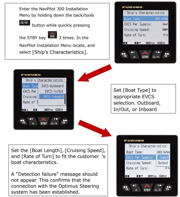
This completes the NavPilot 300 initial settings for use with a Seastar Optimus steering system. Other basic NavPilot 300 settings still need to be set, such as the **Heading source, Position source**, etc.
