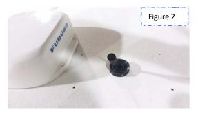
The smaller part of the seal goes into the hole at the top of the roof for which the roof adaptor sits on top of. Then the roof fixture is screwed down the seal makes a tight seal.
