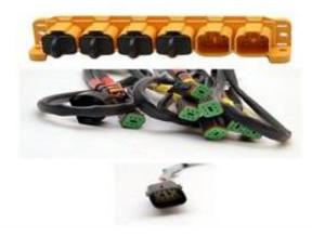
(3) Disconnect the multi-link cable connector and install the Y-split cable for multi link cable installation or if there is a hub simply plug the Yamaha Helm Master gateway into the open port on the hub and disregard the Y-Split Cable. NOTE: There will be several similar style bus connectors but only the correct ones will fit properly.
