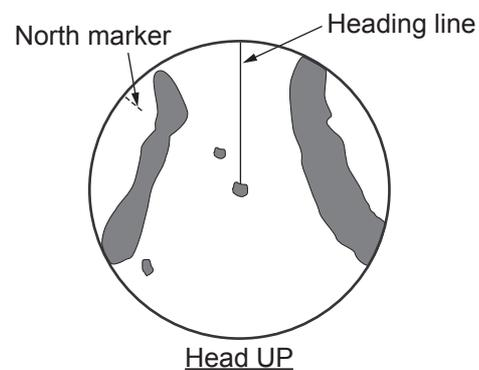
The head-up mode is a display in which the line connecting own ship and the top of the display indicates own ship's heading.
