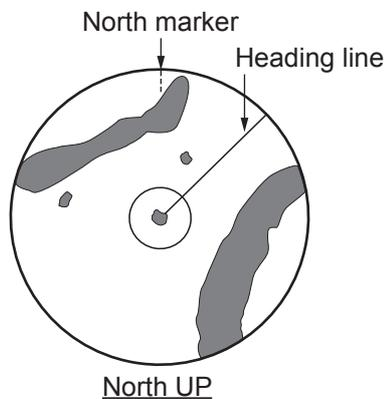
North bearing is maintained at the top of the screen. The heading line changes its direction according to the ship's heading.
