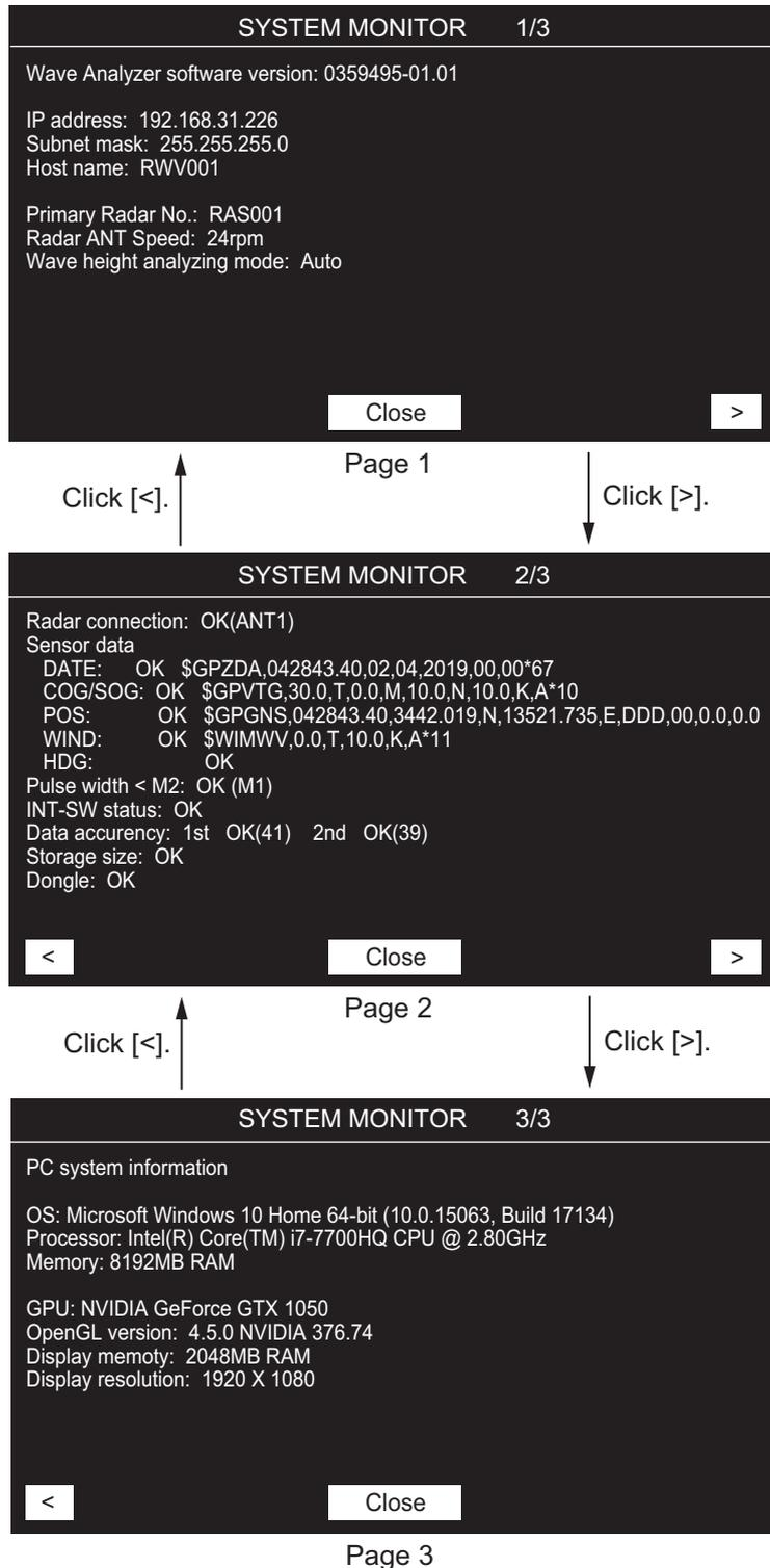
The results for items which fail the system monitor test appear in yellow text with the indication "NG" (No Good).
