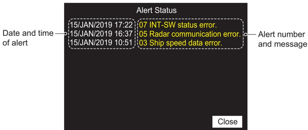
The alerts currently active are shown on the screen. When there is no alert, "No Alert" appears at the center of the screen.
