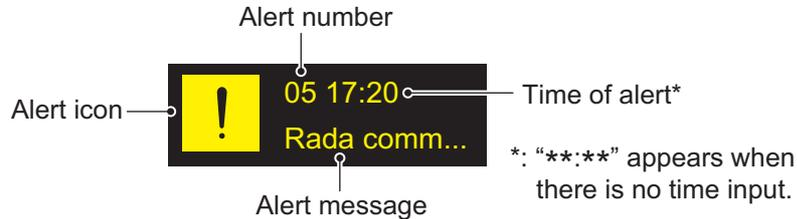
The [Alert Status] displays the number and message of triggered alerts, including the time and date triggered.
