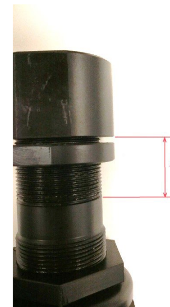
Figure 11. Gland nut travel measurement point for acetal and aluminium glands
