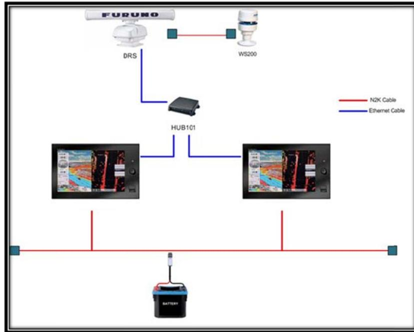
***Note:*** When NavNet 3D and TZtouch are connected on the same Network, this rule does not apply, and the **NMEA2000 backbone should only be connected to the NavNet 3D Master MFD**. Please refer to the “NavNet TZtouch Compatibility” section of this FAQ for more information.
