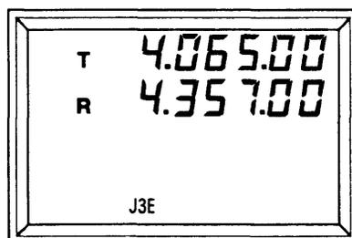
When the antenna coupler could not be tuned, there is no OK display, several beeps sound and "TUNE" disappears.
