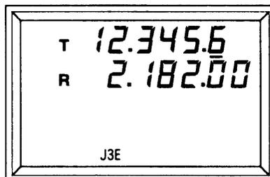
Input frequency with numeric keys.
