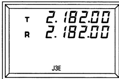
→ When frequencies of radiotelephone are set to 2182 kHz.
