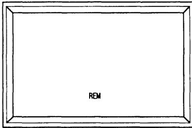
"REM" must appear on the display (handset must be hung) to enable the intercom.
