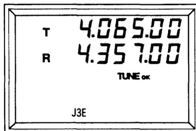
When the antenna coupler is tuned, "OK" appears.
