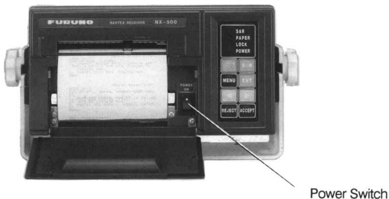
Fig. 2-3 NX-500, Panel opened to show Power Switch
