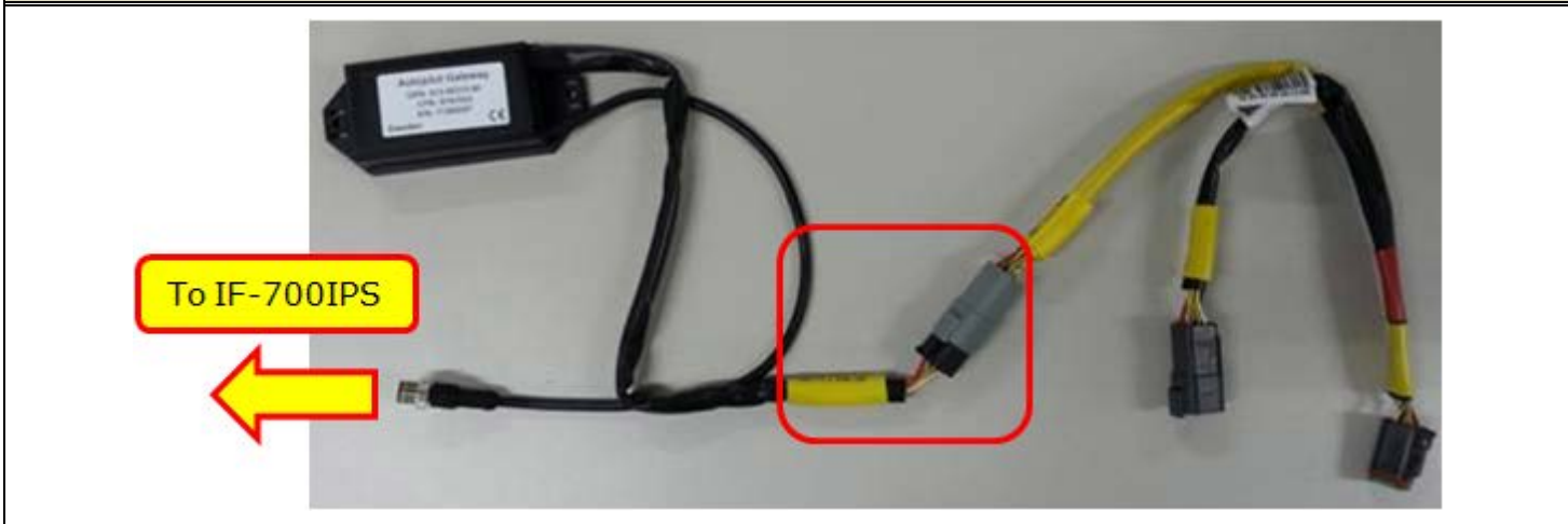
Y-split cable to be connected to the Autopilot Gateway at installation
