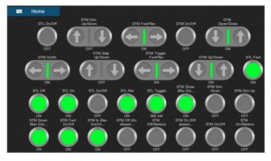
One benefit with the TZTL12F/15F is that both CZone and general <u>NMEA2000 information can be laid</u> <u>out on the same screen</u>. As an example, engine information from general NMEA2000 sensors can be shown in combination with fuel and battery status from CZone.
