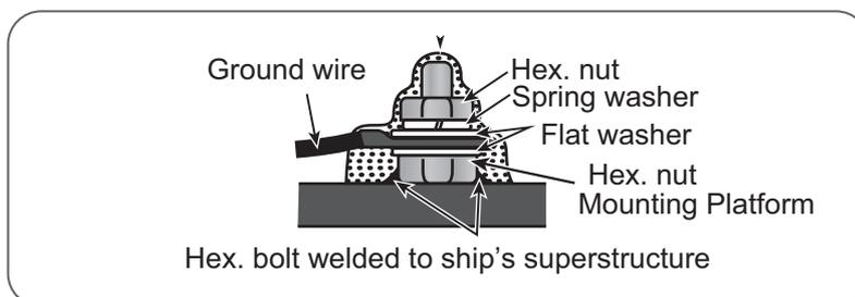
The ground point must be within 300 mm from the ground terminal on the antenna unit.
