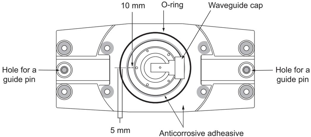
4. Coat fixing holes for the antenna radiator with anticorrosive adhesive.
