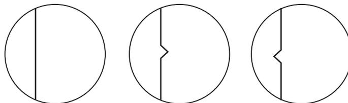
(1) Correct (2) Target pushed inward (3) Target pushed outward
