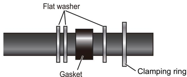
7. Fabricate the signal cable as shown in below.
