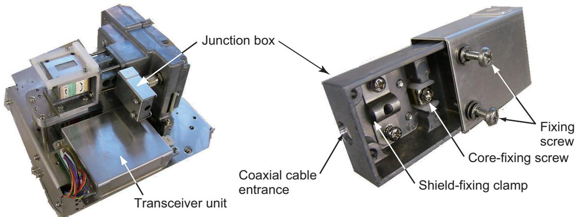
13. Loosen the two screws on the junction box, then slide the cover to open the box. Connect the coaxial cable as shown below.
