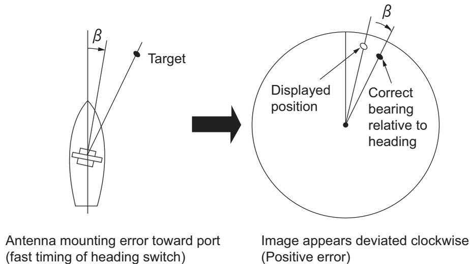
1. Select a stationary target echo at a range between 0.125 and 0.25 NM, preferably near the heading line.
