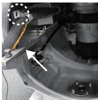
12. Detach the junction box from the transceiver unit.
