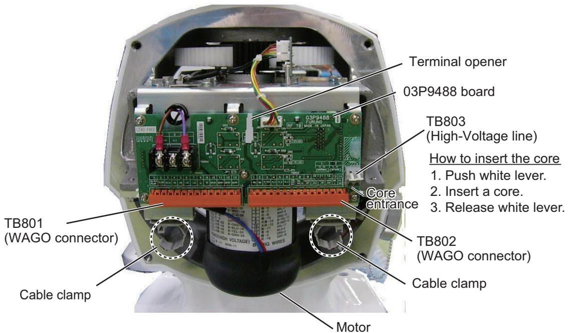
How to connect wires to WAGO connector
