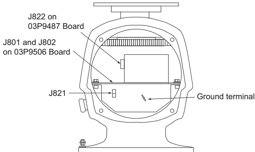
3. Unfasten the transceiver module (two bolts). Remove the transceiver module.
