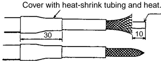
Cut off insulator and core by 10mm.
