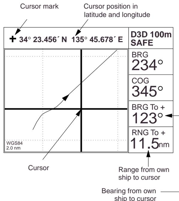
Figure 2-1 Data displayed when the cursor is on
