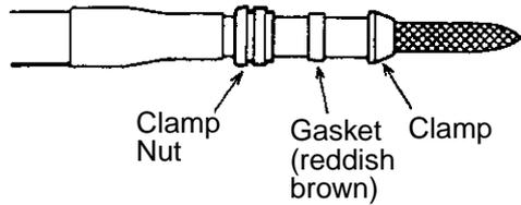
Slip on clamp nut, gasket and clamp as shown left.
