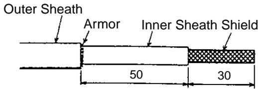
Remove outer sheath and armor by the dimensions shown left. Expose inner sheath and shield by the dimensions shown left.
