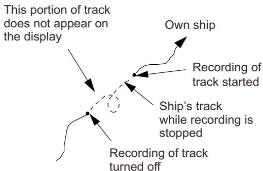
Figure 2-3 Track not plotted or recorded when plotting is stopped
