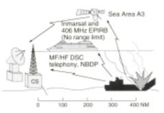
The GMDSS vessels carry the communications equipment appropriate to the Sea Area in which they are operating. Having the capability to choose a long range method when necessary, a call for assistance can reach a coast station and will have a greater chance of being heard by other ships.
