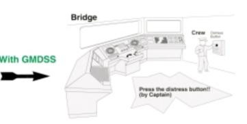
GMDSS equipment provides easy operation in an emergency situation just by pressing the distress button on Inmarsat Maritime MES or DSC. In addition, a float-free EPIRB automatically transmits a distress alert and location.
