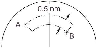
**Note:** If you wish to create an auto acquisition area having a 360-degree coverage around own ship, set point B in almost the same direction (approx.  $\pm 5^\circ$ ) as point A and press the ENTER key.
