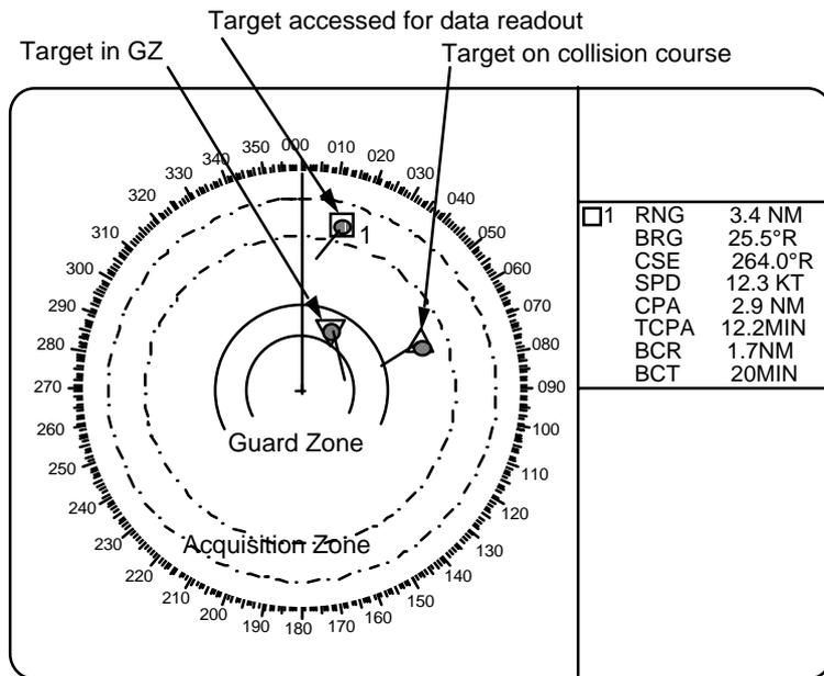
Target being accessed for data readout is marked □ 1, 2 ,...etc.
