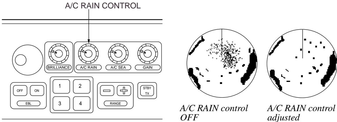
The A/C RAIN control adjusts the receiver sensitivity as the A/C SEA control does but rather in a longer time period (longer range). Clockwise rotation of this control increases the anti-clutter effect.
