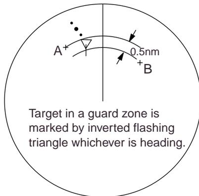
NO. 1 Guard Zone (GZ) is available between 3 and 6 nm with a fixed range depth of 0.5 nm. NO. 2 GZ may be set anywhere when the NO. 1 GZ is valid.
