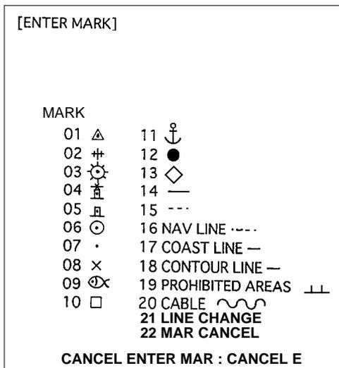
2. Enter mark number to select desired mark, followed by the ENTER key. On the OWN SHIP POSN mode, selected mark is entered to own ship's position.
