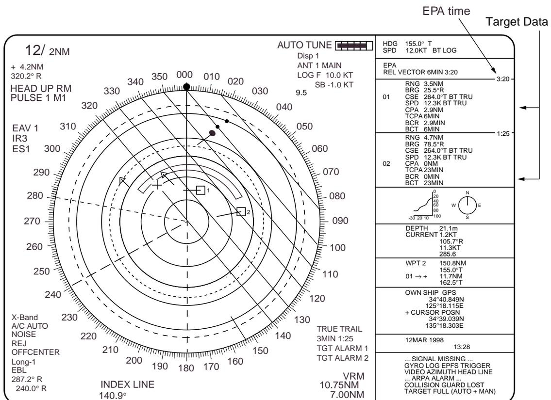
Target 2 is on a collision course as the extension of the vector goes through the own ship position. Placing the offset EBL will be a help for assessment. TCPA is counted up to 99.9 min and beyond this it is indicated as TCPA > 99.9 MIN.
