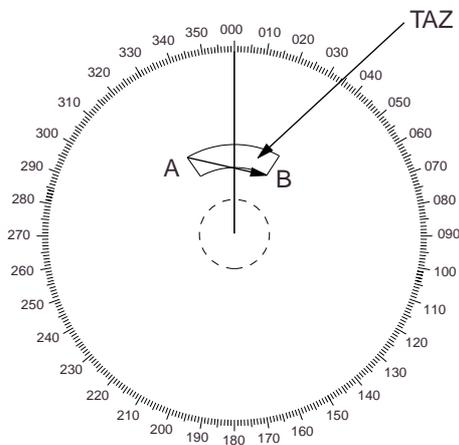
Target alarm zone (TAZ) can be set in any sector between 3 and 6 nm on IMO-type, or anywhere on the R-type.
