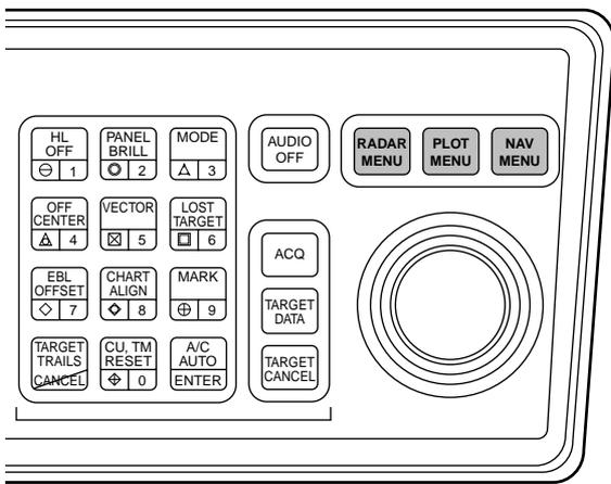
Note: Menu automatically goes off in 30 seconds if you do not press any key.
