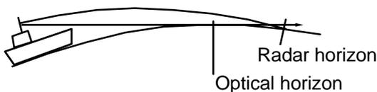
For example, if the height of the antenna above the waterline is 9 meters and the height of the target is 16 meters, the maximum radar range is;
