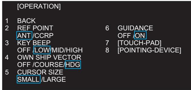
[REF POINT]: The reference point for measurements (range, bearing, etc.) and markers (heading line, stern mark, etc.) can be antenna point or consistent common reference point (CCRP), which is a location on own ship to which all horizontal measurements, for example range, bearing, relative course, relative speed, closest point of approach (CPA) or time to closest point of approach (TCPA), are normally referenced. Select reference point, [ANT] or [CCRP], as appropriate.
