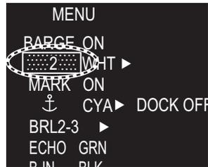
2. Click the [BARGE] icon to enable creation of the barge mark. The cursor shape changes from an arrow to a cross mark.
