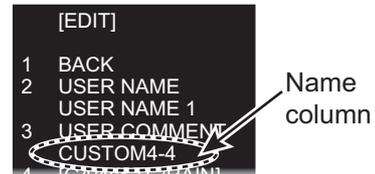
6. To edit the name, press the name column then enter the name with the software keyboard. Click the [END] button to finish.
