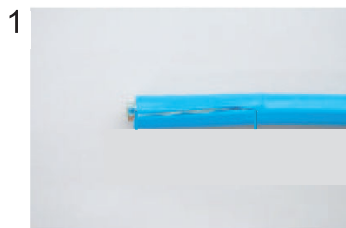
1 Expose inner vinyl sheath.
