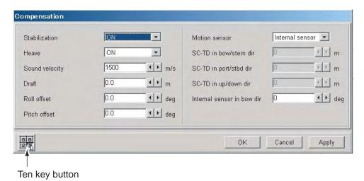
2. Set the following items. To enter numeric values, press the ten-key button at lower left-hand side to open the ten-key panel. Click appropriate numeric keys.
