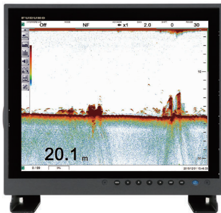
Main monitor: Echoes from FCV-2100 fish finder displayed.
