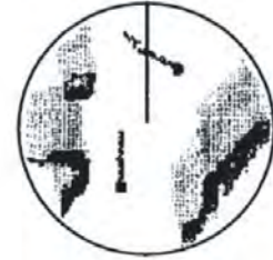
(b) Relative target trails Target moving relative to own ship
