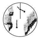
Relative target trails - Targets move relative to own ship, stationary targets are smeared.
