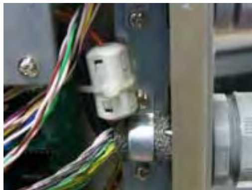
Attaching EMI core RFC-4
