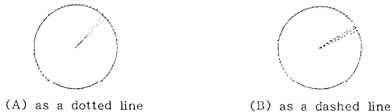
Fig.50 Ramark Signal Appearance
