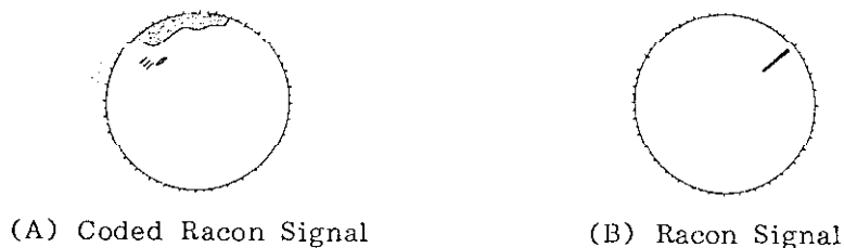
Fig.49 Racon Signal Appearance
