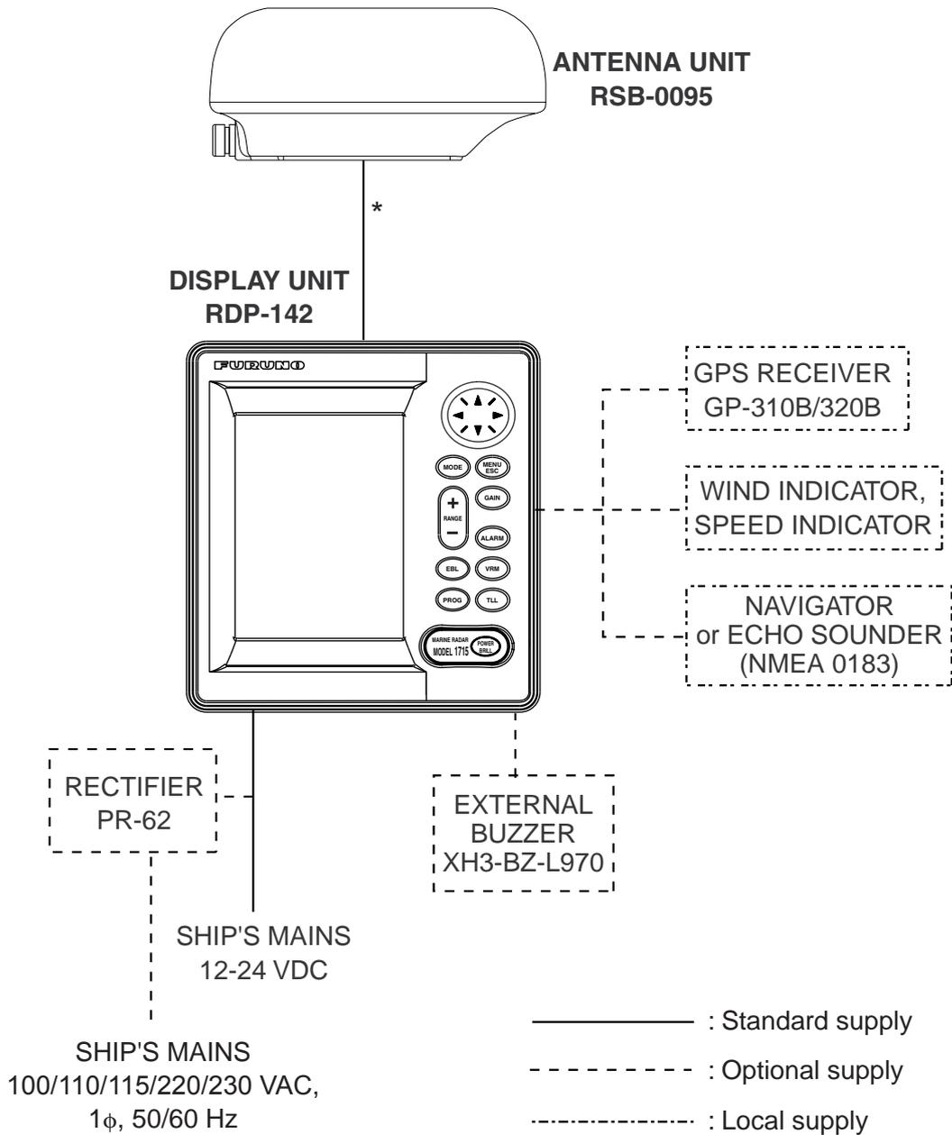
\*: The optional 30 m antenna cable is available for 24 VDC ship's mains only.
