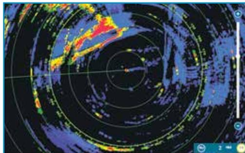
Company A's satellite compass fails to uphold a steady heading, making echo trails virtually unintelligible.
