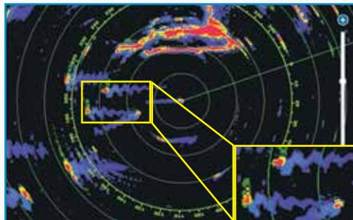
Company C's heading accuracy fluctuates by +/- 5° with a faster update, causing an echo trail that is indistinguishable and confusing.
