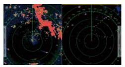
Bird mode and navigation mode can both be displayed via a simultaneous dual mode scanning. Possibility to track the birds while navigating safely \* DRS X-Class Series
