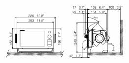
$\begin{array}{ll} \textbf{Multi Function Display (Flush Mount) TZT9} \\ 4.5 \ \text{kg} & 9.9 \ \text{lb} \end{array}$
