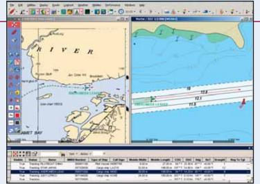
When MaxSea or MaxSea-NavNet is connected to an AIS receiver, you will be able to track multiple AIS targets to gather information on each vessel. Use your PC keyboard as an MKD to send an AIS message to other AIS equipped vessels.
