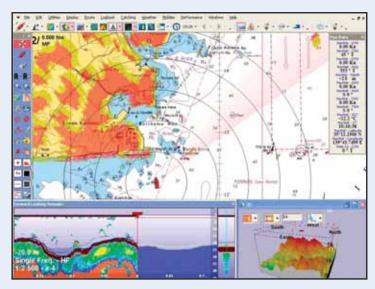
With MaxSea-NavNet you can bring NavNet network information directly onto your PC. This split screen display shows radar targets being overlayed onto a chart, a Forward Looking Depth Profile and a 3D presentation of the seabed.
