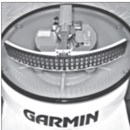
Above: To achieve a lower profile, the Garmin radome's circuit board rotates around the guts of the radome instead of on top of it.
