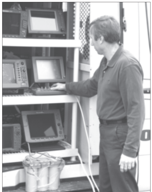
Above: Performance tests included how well each radar showed shoreline 15 miles away and two lobster pot floats 200 yards away.
