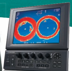
CH300 DUAL-FREQUENCY SEARCHLIGHT SONAR
